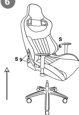
To prevent possible squeaking, we recommend that you secure the plastic O-rings between seat **B** and mechanism **C**, securing them with bolts
